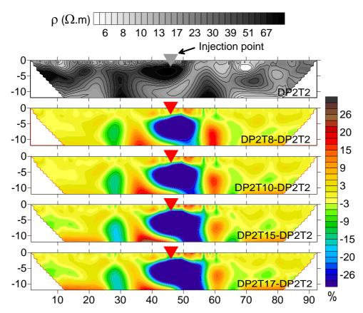
Graph 1 : Preliminary ERT study of the plume of the recirculation system: Interpreted resistivity variations compared with an electrical imaging before the beginning of injection
