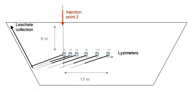
Graph 2: Plot of the lysimeter set-up (cluster B)
