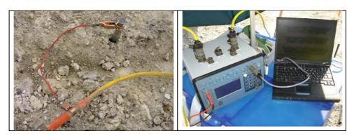
Picture 1: Experimental set-up of the ERT measurement
