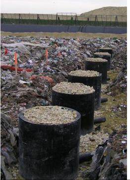
Picture 2: Lysimeters set up in the landfill cell
